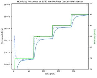
This left plot shows the characterization of a PMMA fiber sensor (no Housing), in a 20°C temperature-controlled environment. With simple signal processing humidity level can be predicted in minutes (dotted line).
