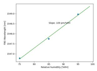
The plot on the left shows the linear relationship between nm change and RH%.
